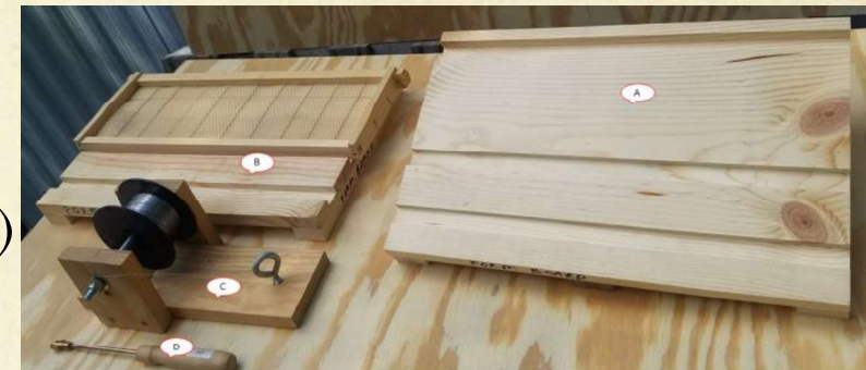
Tools Used to embed horizontal wire into foundation Pictured Items: A. Form board – Commercial supplier versions have a fourth dado cut which is made for shallow frame that isn't widely used any more, so in my homemade version I don't have it. B. Form board with a honey super placed on it. NOTE: Wipe mineral oil on the wood prior to using the form. The oil acts as a release agent to keep beeswax from sticking to the board. C. Cross wire dispensing jig. Homemade item that has a wood wedge on top of the board to apply resistance to the wire spool. D. Small head grooved wire embedding tool (the best version). Large head embedding tools easily slip off the cross wire and don't have the groove in the tool head. Technique: I only use metal wire on honey super frames. I use 15 pound fishing line cross wires for brood chambers, so I can cut out queen cells if they happen to be on top of a horizontal wire. I then put the queen cell in a needy hive or make splits with the queen cell.
